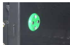
Moisture sensors located inside bale chamber.
