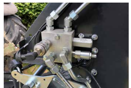
Electronic bale density control.
